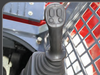
Pilot Operated Controls
