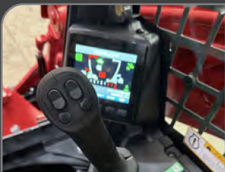
Pilot Operated Controls
